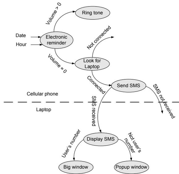
Figure 4. Transition diagram of scenario 3.
