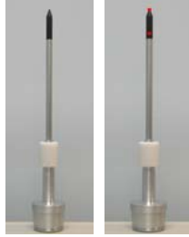
Figure 1. The pathfinder: The tip is made in plastic with two X-ray opaque gold fiducial markers embedded.
