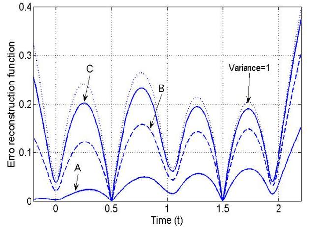
Fig. 6. Error reconstruction functions of a first order RC filter, with nonstationary variance, and the presence of jitter.
