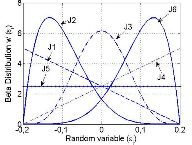
Fig.1. Different jitter pdf. In this case, the distributions are within the symmetric interval  $[-0.2; 0.2]$ .
