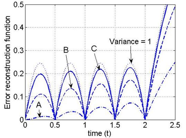
Fig. 4. Error reconstruction functions of a first order filter for some different intervals of variance.
