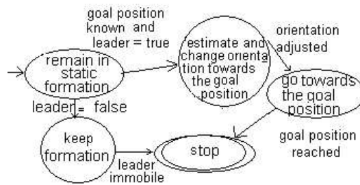
Fig. 3. General algorithm to keep formation . The state keep formation is instantiated according to the agent model (see Figure 4)
