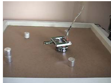
Fig. 8. The Khepera robot set in the middle of a squared arena with simulated food (wooden-cylinders)
