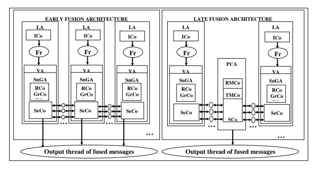
Fig. 1. Principles of early and late fusion architectures (A: agent, C: control, Co: component, Fr: fragments of signal, G: generation, Gr: grammar, I: interpreter, L: language, M: management, P: parallel, R: redundancy, S: semantic, Se: serialization, Sn: sentence, T: time and V: vocabulary). More connections (arrows that indicate the data flow) could be added or removed by the agents to gather fusion information
