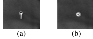
Fig. 1. (a) Head of bolt selected as its essential part. (b) Hole of washer selected as its essential part.
