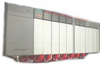
Fig-2 a large PLC
