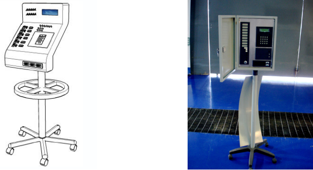
Fig. 2. Engine simulator manufactured to diagnose ECMs.
