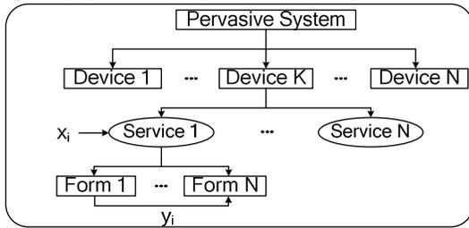
**Figure 1.** Components of a pervasive system: The change in value of  $x_i$  will trigger service1. The change in value of  $y_j$  will change the form of service.
