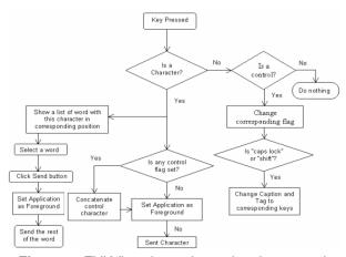
Figure 5. ZVK flowchart when a key is pressed
