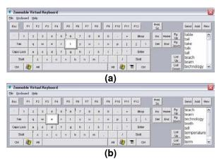
Figure 7. ZVK (a) after typing 't', (b) after typing 'te'
