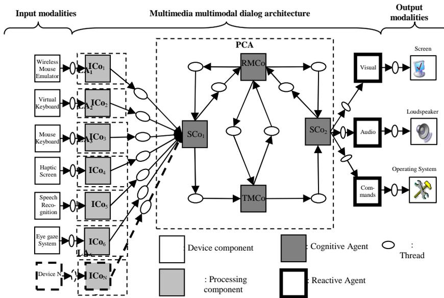
Fig. 2. Multimodal multimedia dialog architecture (A: agent, C: control, Co: component, G: generation, Gr: grammar, L: language, M: management, P: parallel, R: redundancy, S: semantic, T: time and V: vocabulary).
