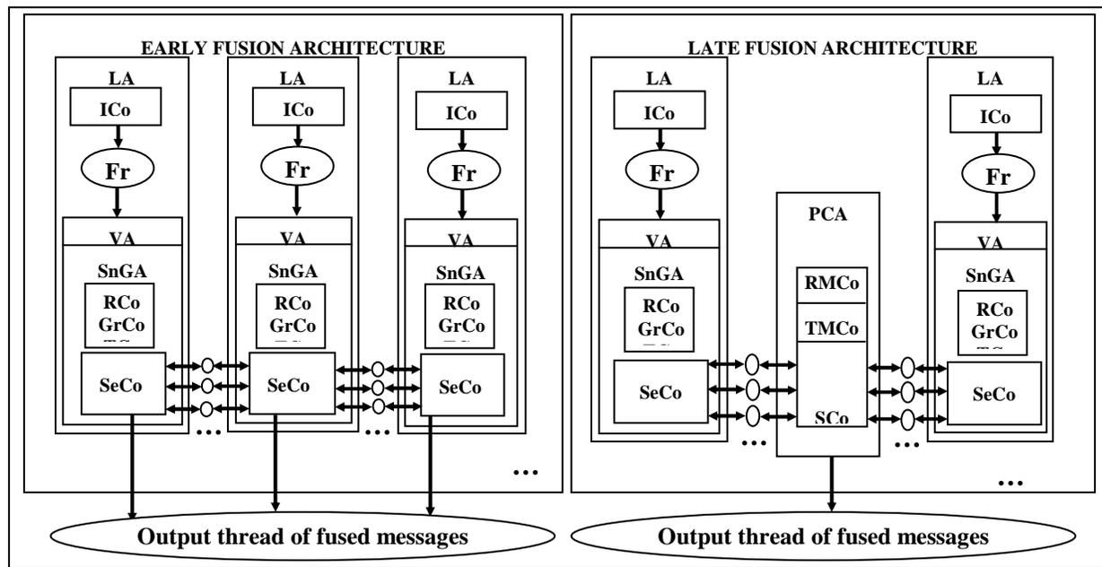
Fig. 1. Principles of early and late fusion architectures (A: agent, C: control, Co: component, Fr: fragments of signal, G: generation, Gr: grammar, I: interpreter, L: language, M: management, P: parallel, R: redundancy, S: semantic, Se: serialization, Sn: sentence, T: time and V: vocabulary). More connections (arrows that indicate the data flow) could be added or removed by the agents to gather fusion information
